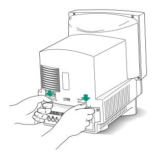
6. Press down on the tabs and pull gently until the back panel opens.
